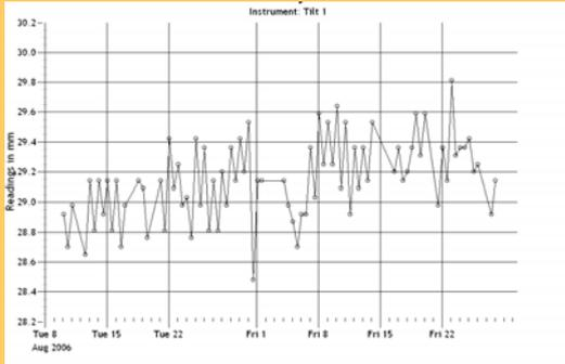
First, we can see the damage is more likely to be due to root induced clay shrinkage, than embankment failure because we have recovery, but the amount of recovery will be a determining factor.
