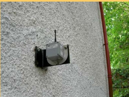
It is important to ensure the sensors are installed in a location, and at an orientation, to capture any movement that takes place.
