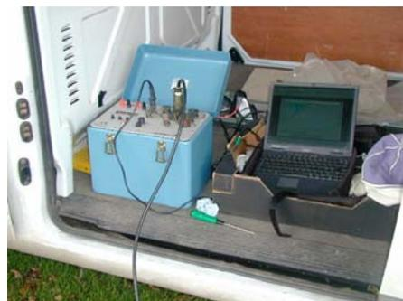
Left we see the ER kit, with readings being taken from a laptop computer between probes cycling through various permutations of spacing to provide values at depth. Thanks to Gary Strong for the snap.
