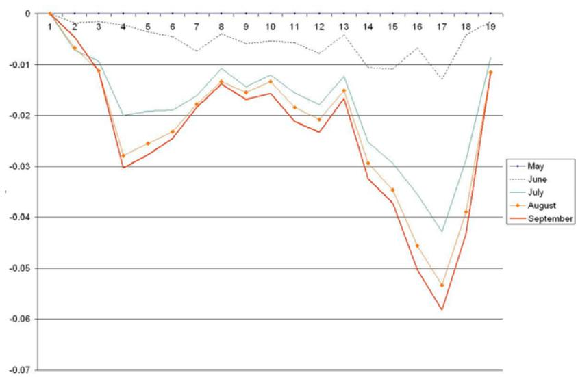
The levelling stations are at 2mtr ctrs, and the total distance between extreme stations (No's 1 and 19) is 38mtrs taking account of the gap between centres at the position of the trunk.
